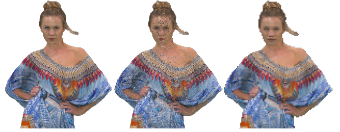
Fig. 1: Downsampling approaches. Original PC (857,966 voxels), set downsampling (64,176 voxels D1_{PSNR} = 61.5\text{dB} ), and grid downsampling (62,130 voxels, D1_{PSNR} = 58.4\text{dB} ).
