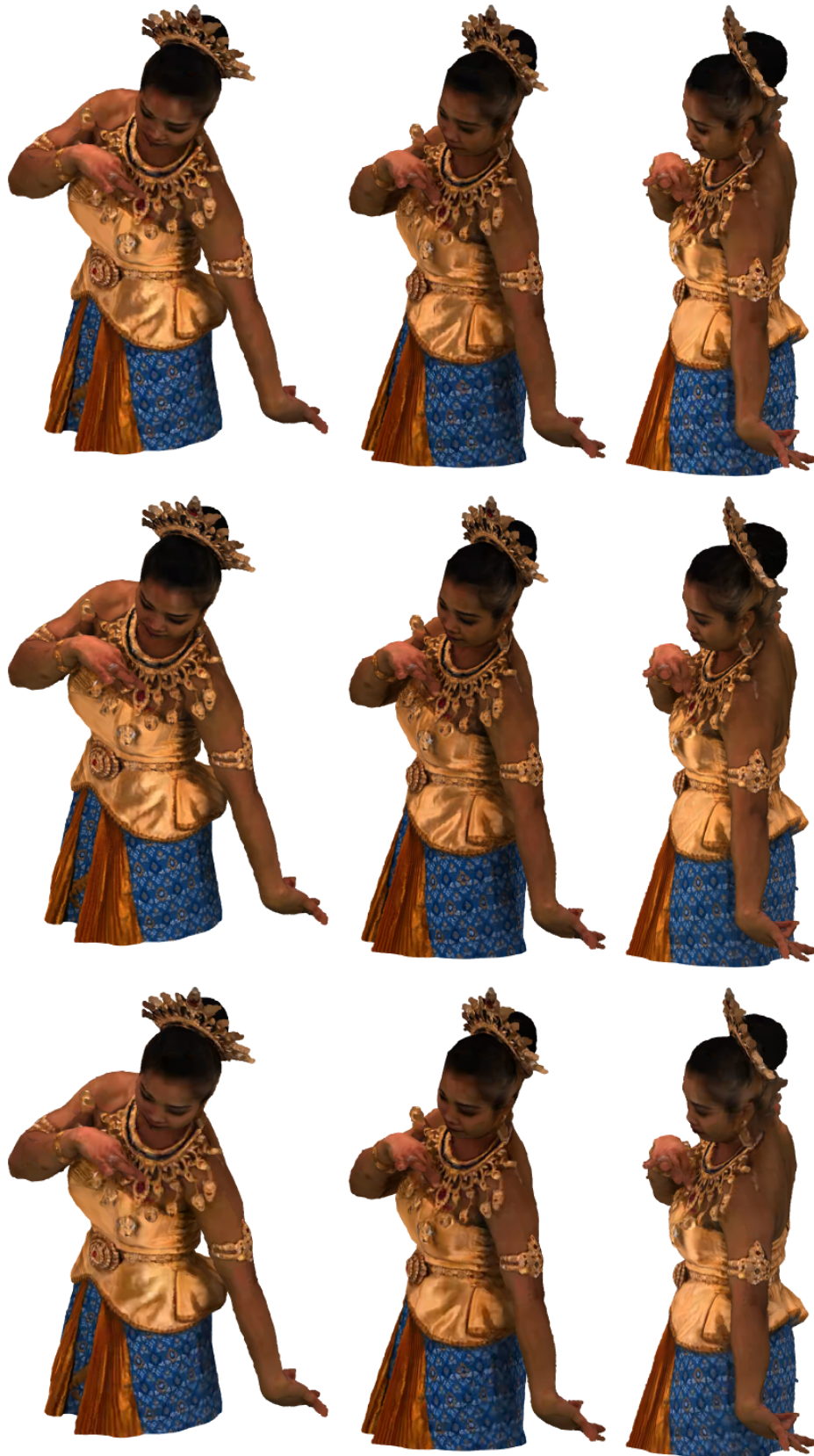
Figure 15. Decoded views (cameras 5, 6 and 7) of the plenoptic Thaidancer PC. First row: V-PCC, where the plenoptic data occupies 8488000 bits, or 9193136 bits when considering the default RGB value triplet rgb , in both cases with a PSNR of 34.5 dB with respect to the original point cloud. Second row: plenoptic differential coding, where the plenoptic data occupies 968080 bits when considering rgb , with a PSNR of 34.3 dB. Third row: plenoptic non-differential coding, where the plenoptic data occupies 876160 bits, with a PSNR of 34.1 dB.
