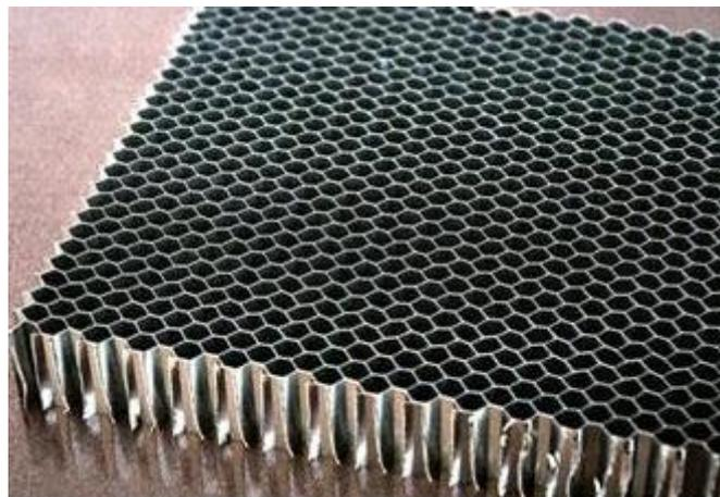
Figura 24: Estrutura hexagonal de *Honeycomb* [ALUSTRONG, 2016]
