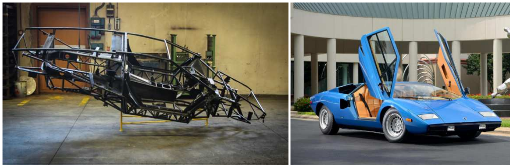
Figura 12 - Chassi tubular Lamborghini Countach
