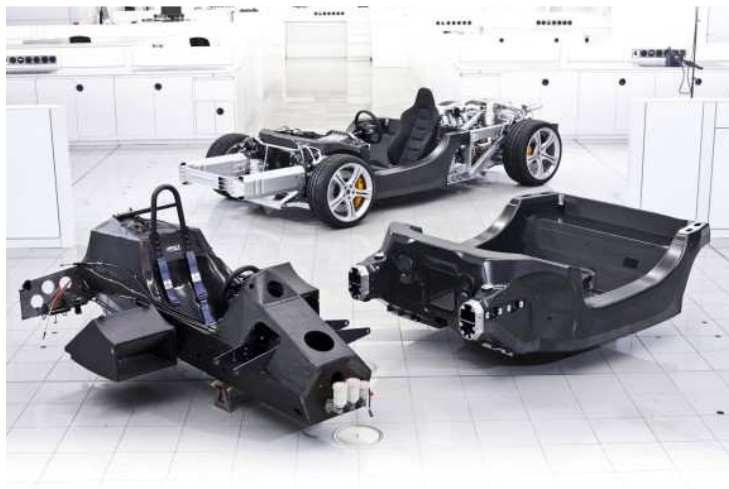
Figura 14 - Chassis monocoque McLaren Racing
